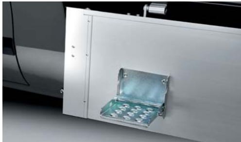
Internal steps folding into sideboards
