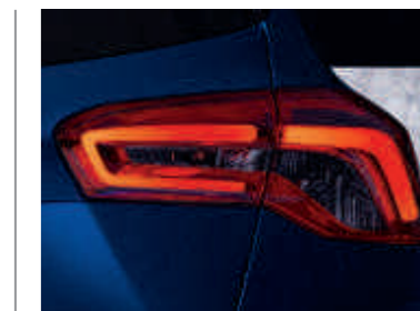
LED/Halogen LED/halogen rear lights incorporate an LED signature strip which illuminates when the headlights are switched on. (LED rear lights are standard on Titanium and Vignale; halogen rear lights are standard on all other series)
