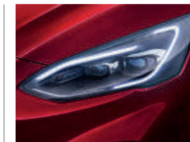
Adaptive Front lighting System with dynamic LED headlights, glare-free high beam and LED sequential turn indicators (Option)
