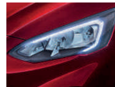
Halogen headlights with LED daytime running lights (Standard)
