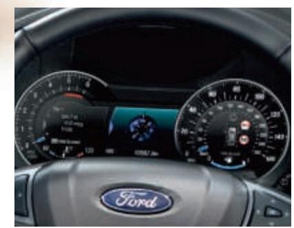
10.1" colour TFT cluster display (Standard)
