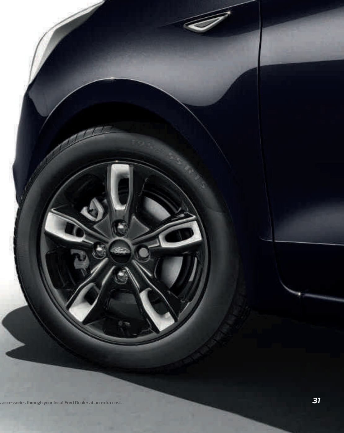
15" 8x2-spoke steel wheel (Fitted with 195/55 tyres) Sd
