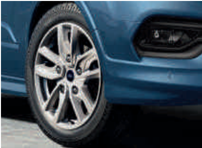
18" alloy wheels with 235/50R18 tyres (Option on Van. When fitted, vehicle is designated as a 290 model) (N/A for ROI)
