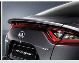
Trunk lid with spoiler effect To improve stability and optimise airflow that forms behind the Stinger when travelling at higher speeds, the trailing edge of the trunk lid is arched, providing a spoiler effect – and a stunning finale to the Stinger silhouette.
