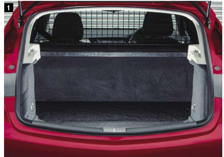
1. Load area. Providing a completely flat inner load floor area that combines a maximum load length of 1550mm with a maximum width of 1350mm.
