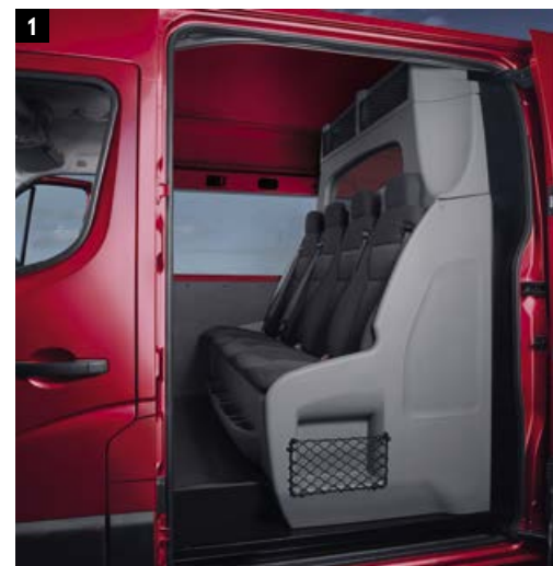
1. Room for all the crew. The Doublecab features four individually contoured rear seats with lap and diagonal seatbelts. Rear storage includes a full-length tray under the seat cushion, plus optional overhead and side net pockets.
