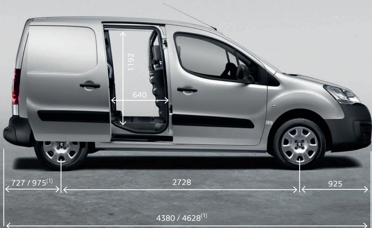
The Peugeot Partner comes in two different lengths, which means two loading volumes and lengths. The Standard panel van is 4380mm long and the Long Body panel van is 4628mm long, to deliver a load floor length
