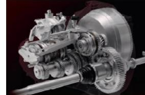
Exclusive to PEUGEOT 308 GTi 270 by PEUGEOT Sport is an accomplished Torsen® limited-slip differential, incorporated into the transmission to improve cornering traction. By channelling the torque to the wheel with the most grip, it allows the car to accelerate faster as it exits bends than would normally be the case.
