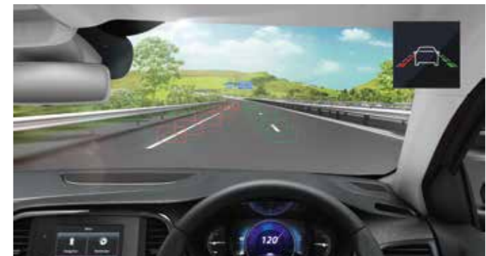
Lane departure warning: (1) This system detects the lane in front of the vehicle with a camera and warns the driver audibly if they drift into another lane .
