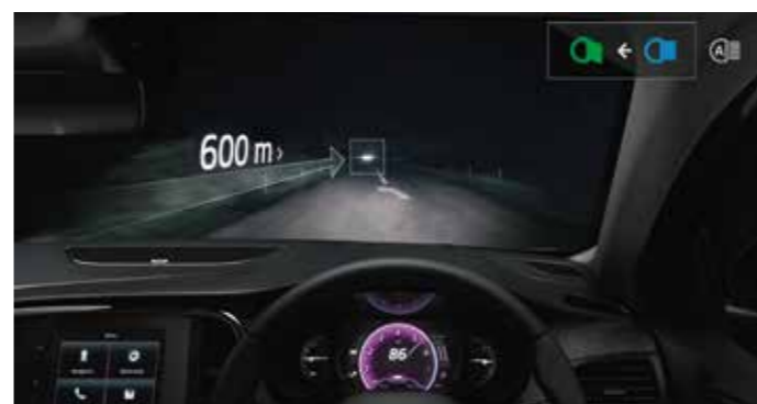
Auto high/low beam: (1) High beam automatically switches to low beam when the front camera detects other vehicles around and automatically switches back to high beam when nothing is detected around.
