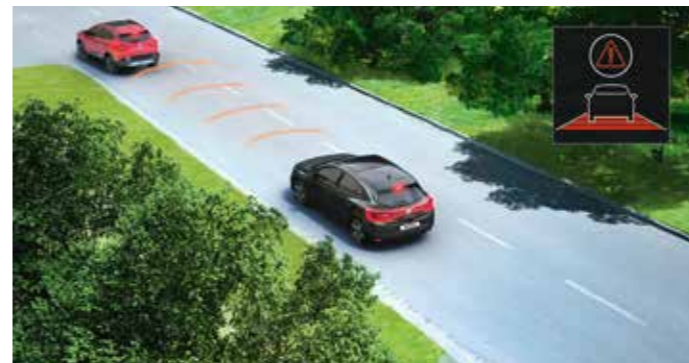
Active emergency braking system: (2) This system alerts the driver if there is a risk of collision with the vehicle in front. If the driver reacts insufficiently or not at all, the brakes are activated to prevent or mitigate a collision.
