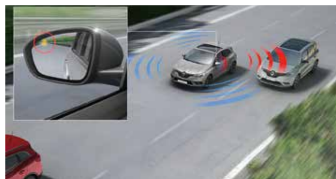
Blind spot warning (3) Expand your vision! New Renault Mégane is equipped with a system which detects the presence of any vehicle in the zone that your wing mirrors do not allow you to see. Active between 19 mph and 87 mph, the system alerts you straight away with a warning light.
