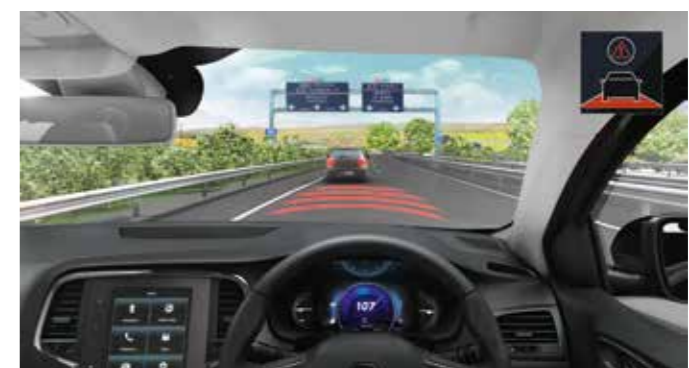
Safe distance warning: (2) This system warns the driver about potential collision with another vehicle in front, if the distance between the vehicles is not safe.
