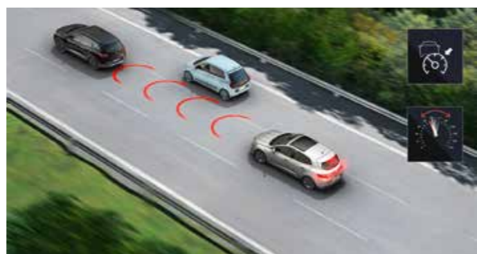
Adaptive cruise control (3) Easily maintain the appropriate safe following distance between you and the vehicle in front. In order to adapt your speed, the adaptive cruise control is activated at between 50 km/h and 140 km/h. The system acts on the brakes when the distance is too short and on the accelerator when the road is clear again.
