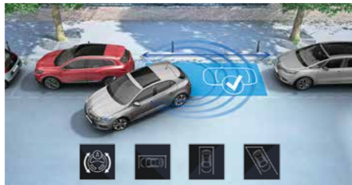
Hands free parking (3) Parallel parking with a flick of the wrist! Hands free parking helps you to identify the parking space configuration (parallel, diagonal or perpendicular), measures the available space and handles the manoeuvre. All you have to do is control the accelerator, brakes and gears. A genuine co-pilot by your side!
