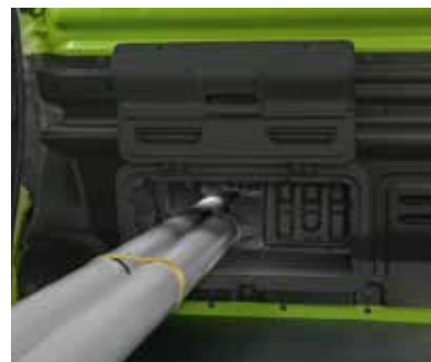
Load through bulkhead flap is magnetised to fix easily and securely in place
