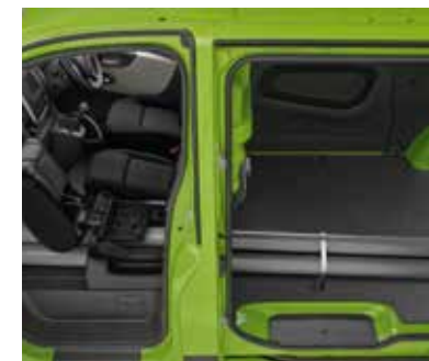
Load through bulkhead allows you to load in to passenger foot well
