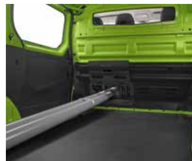
Load through bulkhead flap is magnetised to fix easily and securely in place
