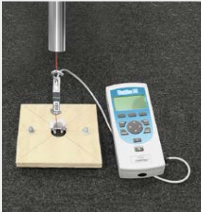
Testing of fixing element strength
