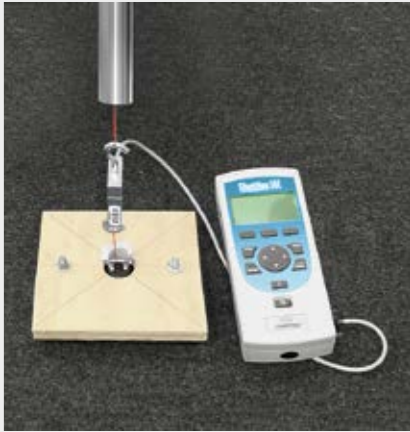
Testing of fixing element strength
