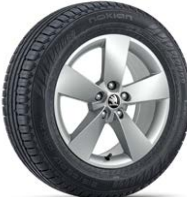
Ratikon 565 071 497A 8Z8 light-alloy wheel 7.0J x 17" for 215/65 R17 tyres ET40, silver metallic ŠKODA Genuine Accessories
