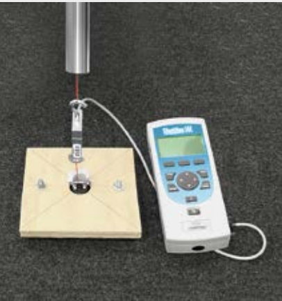
Testing of fixing element strength
