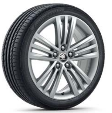
Trinity 3T0 071 498J 8Z8 light-alloy wheel 7.5J x 18" for 225/45 R18 tyres ET46, silver metallic (only for OCTAVIA SCOUT) ŠKODA Genuine Accessories
