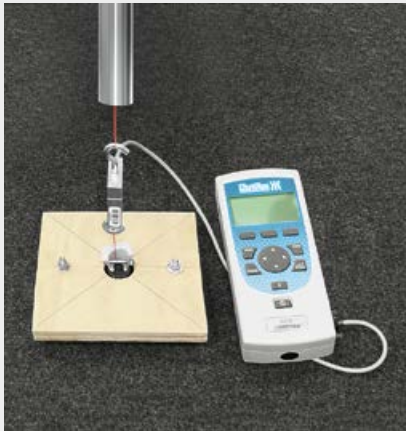
Testing of fixing element strength
