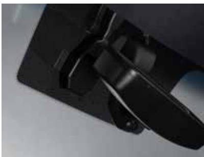
Front camera module with rain-sensing and automatic light control unit
